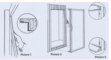
sides is somewhat concave/oval in relation to the door straighten it with the aid of a shim or similar between the door and the frame side or between the element and door frame. Allow the door frame with door closed to harden for a minimum of 8 hours with the door and frame in the correct position, without putting strain on the openings. If necessary, the hinges can also be adjusted sideways by loosening the hinges in the frame with a 4 mm Allen key.
